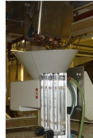
The Ultra Slim Stealth Vertex metal detectors screen a variety of nuts prior to bagging at speeds of 80 packs per minute
