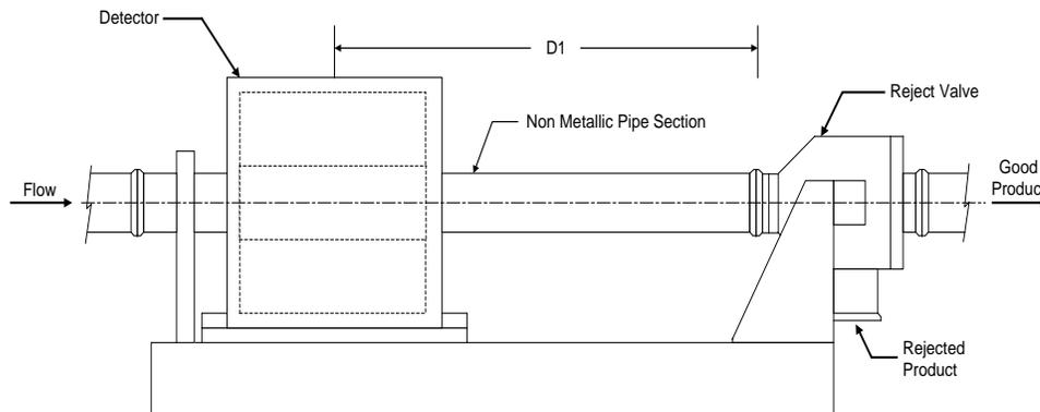
The pipeline application involves the installation of a non-metallic pipe section around which a metal detector inspects products travelling through the pipe. This type of application should be considered where the extra sensitivity capability of a relatively small aperture outweighs the benefit of final package inspection. This is especially true if the final packaging material contains metal, such as a canning line.
