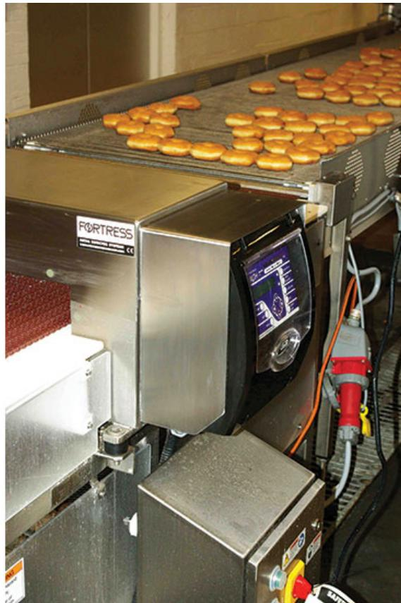
Doughnut Peddler installed Stealth conveyor systems on its production lines, with each capable of checking 160 doughnuts per minute.
